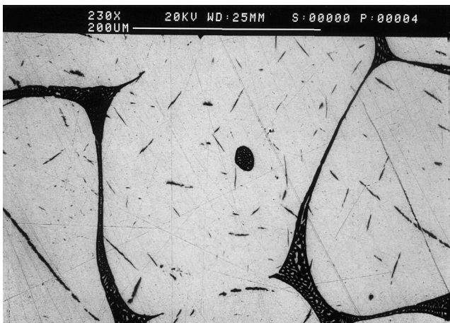
Fig. 7. BSE micrograph of Gd-5.0 at% Cu alloy, melted and cooled in DTA equipment at 5 K/min. Primary crystals of (Gd) surrounded by eutectic structure ((Gd)+GdCu). A typical drop of catatctic liquid, showing the subsequent eutectic reaction, can be noticed inside the central crystal.
